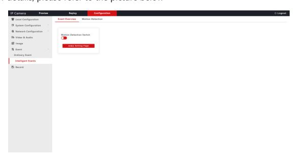
(2) Enable Motion Detection (The device detects moving objects in the area)
